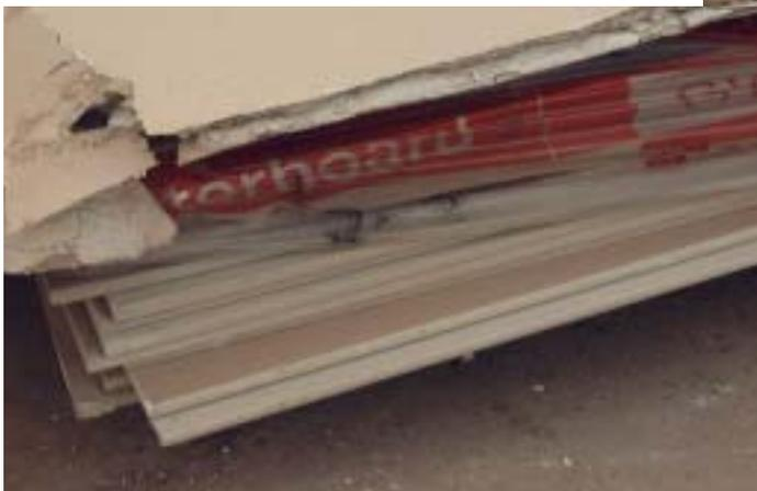
*Figure 15: An example of packs that have become fully exposed.*
