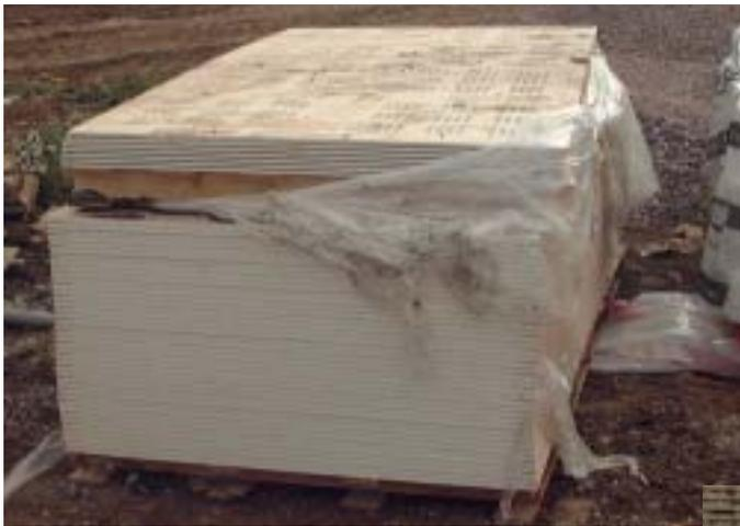
*Figure 13: An example of poor covering of packs after splitting of the shrinkwrap.*
